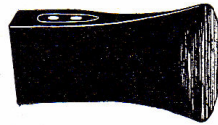
Fig. 14.—Incorrect grind. Too steep a bevel and file marks run along the edge back toward the head.
