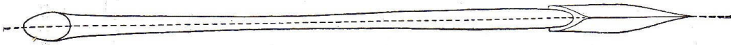
Fig. 16.—In a correctly hung axe, the cutting edge is in a direct line with the center of the handle.
