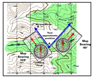
and repeat the process: you are somewhere in the triangle formed by these three lines. To be more accurate, take more bearings and trace them onto the map.
